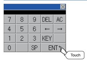
**3.** The keyboard for entering a keyword is displayed. Enter a keyword and touch the [ENT] key. Character types to be input can be changed by touching the [KEY] button.
