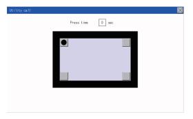
1. Touch or displayed at the four corners of the setting screen. The button repeats every time it is pressed. Change the part to be set as a key position to . For the key position, 0 or 1 point can be specified.
