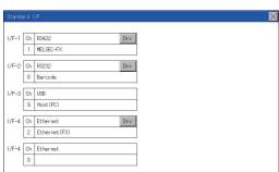
**3.** When the channel number is selected, the settings are fixed and the window returns to the previous one. Therefore, touch the [x] button.
