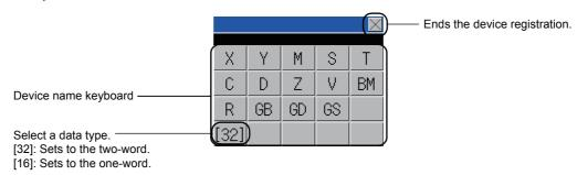
8 9 A В 4 5 6 C D Device number keyboard 1 2 3 Ē F 0 AC DEL (ENT) Deletes all input numbers. Registers the input device. (The device registration is completed.) Ends the device registration.
