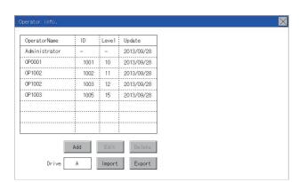
**3.** When the administrator password is correctly input, the Operator information management screen is displayed. For operation of operating switches, refer to the following.
