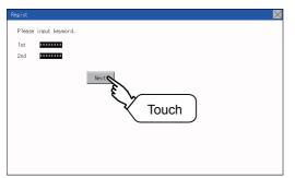
**5.** After completing the keyword entry, touch [Next]. When [Keyword+Custom] is selected on the selection screen for the registration, the Customer Keyword entry screen is displayed. Enter it in the same way as for Keyword and 2nd keyword.
