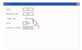
**2.** If you select [Sampling], set the sampling interval for the clock adjustment. Touch the entry box on the left side of [Min.] to display a software keyboard. Input a value with the keyboard.
