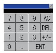
(a) Touch [Auto logout time], and then the Auto logout time edit dialog box is displayed. Input the time.When the input is completed, touch the [ENT] key.
