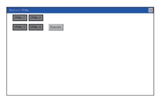
**2.** Select the CPU unit to be restored by pressing a switch (among [CPU No. 1], [CPU No. 2], [CPU No. 3] and [CPU No. 4]). When the connected equipment is an FX CPU, touching any switch (among [CPU No. 1], [CPU No. 2], [CPU No. 3] and [CPU No. 4]) is invalid.
