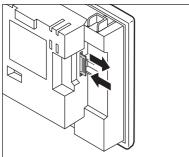
**2.** Push the SD card all the way inside and leave your finger once, then remove the SD card.
