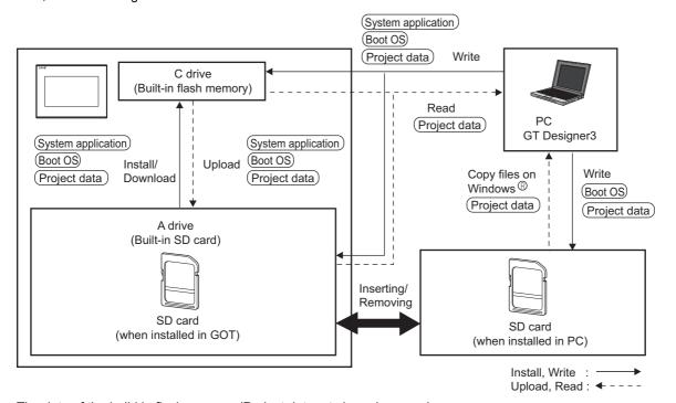
The data of the build in flash memory (Project data, etc.) can be saved.
