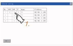
**1.** Touch the Net No. to be changed, and input the network No. to be changed by the numeric keypad displayed.
