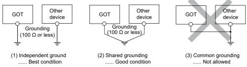
• Use the cable of 2mm<sup>2</sup> or longer for grounding. Make a ground point near the GOT as much as possible to shorten the ground cable.
