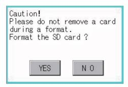
**4.** Type 1 1 1 and touch the [Enter] key. The dialog box shown on the left will appear. (The password is fixed to 1111.) Confirm the contents of the dialog box, and touch the [YES] button to format the SD card. To cancel the format, touch the [NO] button.
