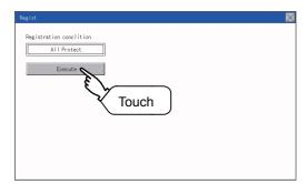
**7.** After setting the registration condition, touch the [Execute] key. The registration of the keyword is completed.
