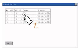
Touch the station No. to be changed, and input the station No. of the destination Ethernet module to be changed by the numeric keypad displayed.
