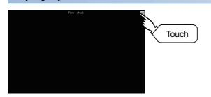
**1.** Touching the [×] key closes the screen. Even if touch points other than the upper left corner and upper right corner of the screen, the GOT does not operates.
