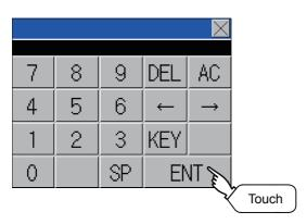
4. The keyboard for entering a keyword is displayed. Character types to be input can be changed by touching the [KEY] button. Enter a keyword and touch the [ENT] key. For the keyword, 8 digits from 0 to 9 or A to F must be set.
