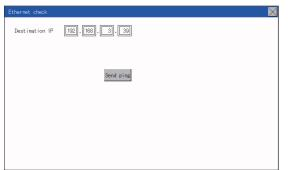
If the select button of [Destination IP] is touched, a keyboard is displayed. Enter the IP address of the other terminal with the keyboard. <Default: 192.168.3.39>
