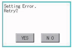
**5.** When the precise touch could not be made, touch the [YES] button to make the setting from Step1 again.
