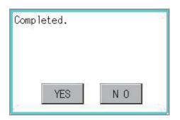
When the administrator password is correctly input, the dialog box shown left is displayed and the operator information stored in the GOT is exported to an SD card. (file name: AUTHINF.G2U)
