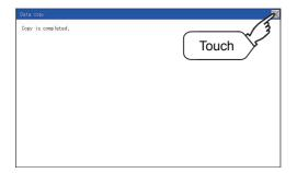
**6.** Copy is completed. If the [×] button is touched, the screen is closed. If an error occurs during copy, an error message appears. For details of error messages, refer to the following.
