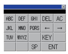
**3.** Input the current password on the Password change dialog box. Character types to be input can be changed by touching the [KEY] button.
