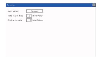
**2.** When the administrator password is correctly input, the Function setting screen in displayed. Touch an item to be set.
