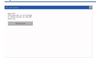
**1.** Touch a setting item to change the setting. [Permissions] [Access inhibit] When installing or removing an SD card, always set [Access inhibit].
