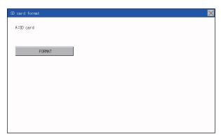
**3.** If touch the [FORMAT] button, the password input screen is displayed.
