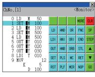
When the list monitor is started on the FX list editor screen, the step numbers displayed on the FX list editor screen is displayed on the list monitor screen.
