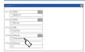
**1.** Touch the driver display box of a communication parameter to be set.
