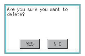
**2.** If touch the [Delete] button, the dialog box mentioned left is displayed. If the [YES] button is touched, the file or folder is deleted. (While executing, [Processing...] message appears on the screen.) If the [NO] button is touched, the deletion is canceled.
