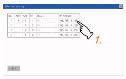
**1.** Touch the IP address to be changed, input the destination IP address to be changed by the numeric keypad displayed.
