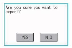
**4.** The dialog box shown left is displayed. When the [YES] button is touched, the Admin password authentication screen is displayed. Input the administrator password. Character types to be input can be changed by touching the [KEY] button.
