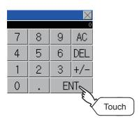
2. When the ten-key pad appears, enter a numerical value in up to 3 digits, and touch the ENT key. If a numerical value outside the setting range is entered, the following error message appears. Enter a numerical value again.
