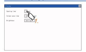
**1.** If the setting items (numbers) are touched, a keyboard is displayed. Input numeric with the keyboard.
