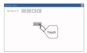
**2.** If the [Send ping] button is touched, a ping is sent to the IP address entered in [Destination IP]. The timeout time is 5sec.
