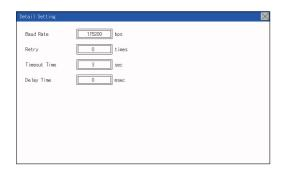
**2.** The screen jumps to the detailed information screen and the communication parameter will appear.
