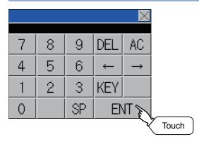
**3.** The keyboard for entering a keyword is displayed. Enter a keyword and touch the [ENT] key. Character types to be input can be changed by touching the [KEY] button.
