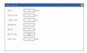
**2.** The screen is switched to the communication detail setting. Set the communication parameter on this screen.
