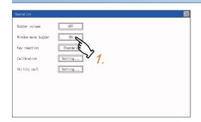
**1.** Touch a setting item to change the setting. (Window move buzzer: ON OFF)
