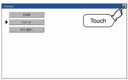
After changing the setting, touch the [x] button. The setting is saved and the setting screen is closed.
