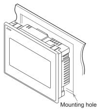
Inserting into the panel face
