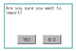
2. The dialog box shown left is displayed. When the [YES] button is touched, the Admin password authentication screen is displayed. Input the administrator password. Character types to be input can be changed by touching the [KEY] button. When the input is completed, touch the [Enter] key.
