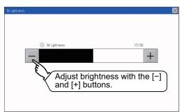
**2.** Touch the [+] and [-] buttons to adjust the brightness of the screen.
