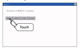
1. Touch "Regist" to display the selection screen for the registration. For the FX series PLC, which is not compatible with Customer Keyword, the keyword entry screen of [Step3] is displayed. Start the operation from [Step3]. For the Customer Keyword compatible models, refer to the manual of the PLC to be used.
