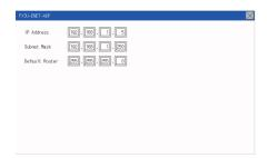
**5.** When the screen shown on the left appears, the changed communication set value of the FX3U-ENET-ADP is written normally to the CPU. For making valid the contents of setting, turn OFF the power of the CPU, and then turn it ON again. Change the setting of the subnet mask pattern and default router IP address using the same procedure if necessary. An error message appears in the following cases. Touch the OK key to return to the step 1., and perform the setting procedure again.
