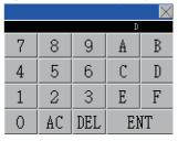
The device registration is completed by touching the [ENT] key.
